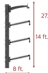
115kV Transmission Spacer Cable
